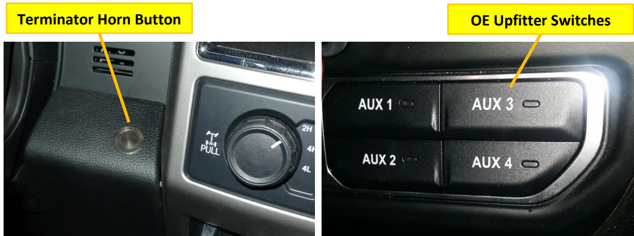
Figure 35 – Horn Button Installed in Dash and OE Upfitter Switches (Shown in example vehicles)
