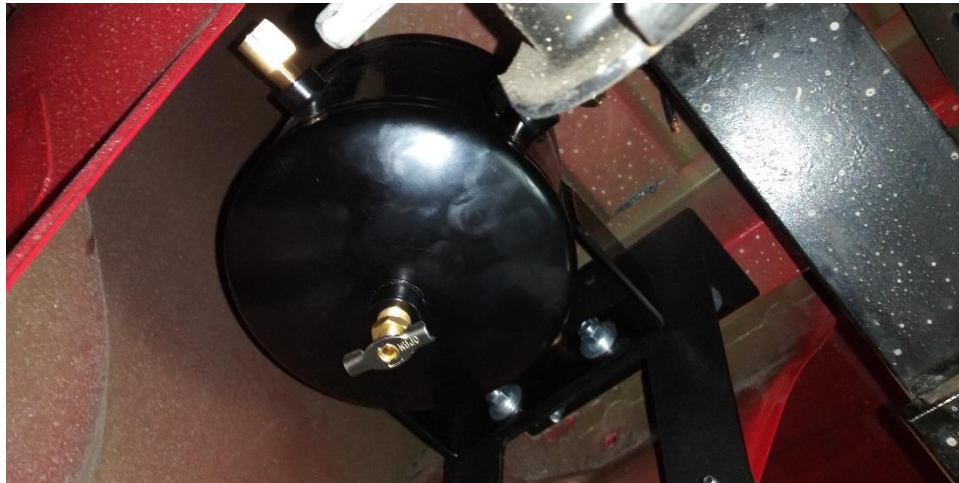
Figure 3 – Under Vehicle view of Air Tank Installed – Behind Driver Bed Side (2020 Silverado Shown)
