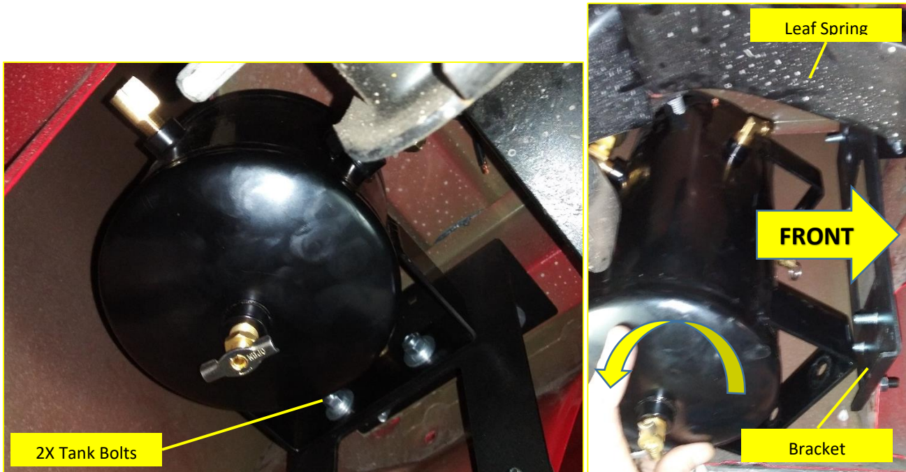
Figure 19 – Installing Air Tank onto Air Tank Bracket (2020 Silverado Shown)
